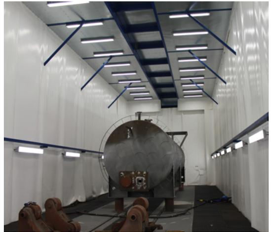
The general view of a blasting chamber with its basic components, based on automatic abrasive collection and regeneration conditions, is presented in the figure below.
